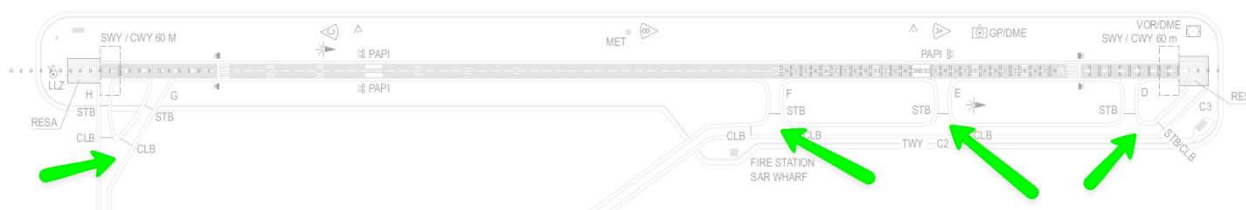
Figure 8.3: The TWR controller shall instruct arrival aircraft to stop at the indicated locations and contact the GND controller. (Source: AIP Macau, AD2-VMAC-52)
